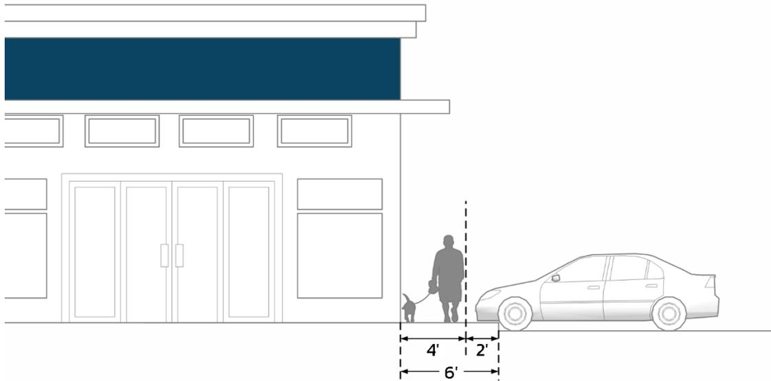
**Figure O4.5: Maximum Vehicle Overhang**
